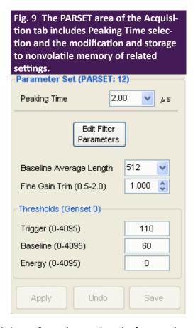
The configuration process needs only be performed once, though of course the parameter sets can later be modified.
